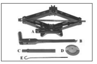
The tools you'll be using include the jack (A), folding wrench (B), extension tube (C), wing nut (D), and J-Hook (E).
